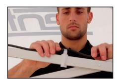
Press the cord down into the top of the plastic clips so that the cord runs neatly across the scissor piece and hangs down on the inside of the chosen leg.
